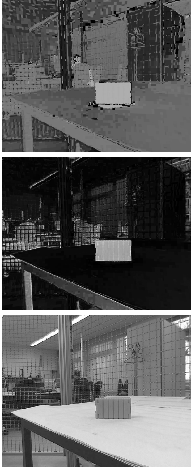
Figure 22.: HSV color space. Top to bottom: the hue, saturation, and value planes of the image in Figure 21.
