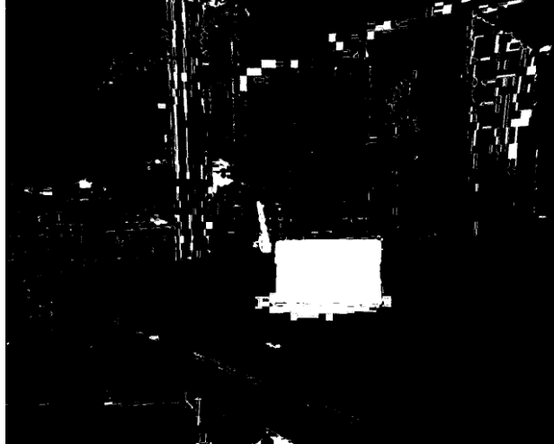
Figure 23.: Hue plane thresholding. The pixels identified as red pixel by thresholding the Hue plane.
